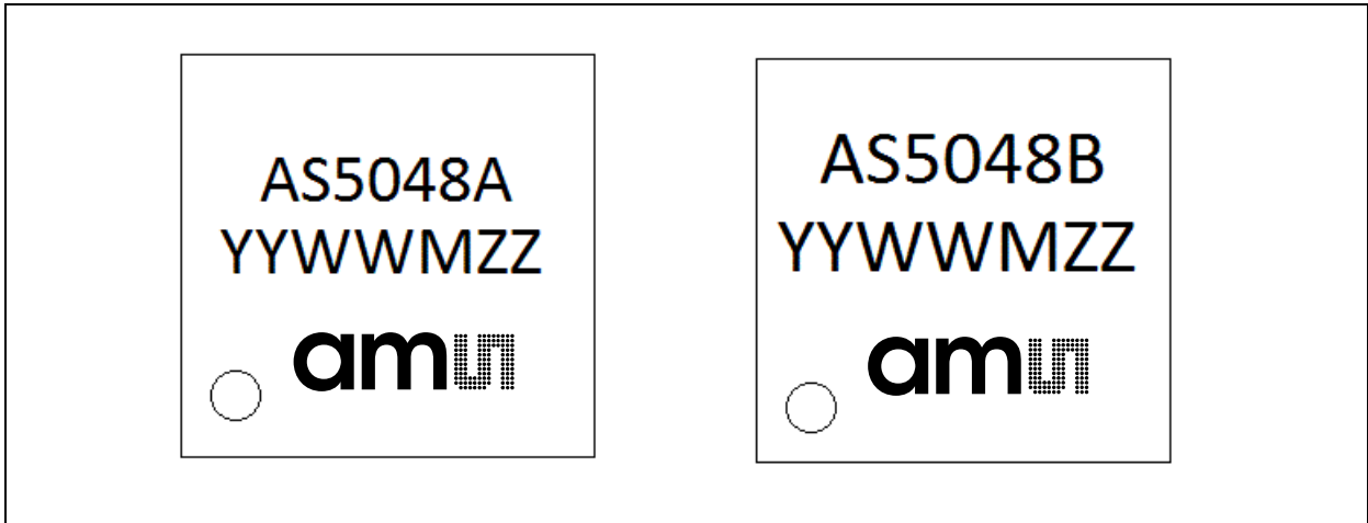
Figure 39: Package Markings for AS5048A & AS5048B
