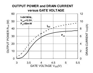
RoHS Compliance, 896-941MHz 20W 12.5V, 3 Stage Amp. For MOBILE RADIO
