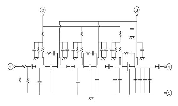
RoHS Compliance, 896-941MHz 20W 12.5V, 3 Stage Amp. For MOBILE RADIO
